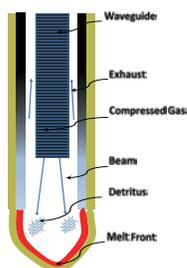
Schematic of Millimeter-wave Drilling System
