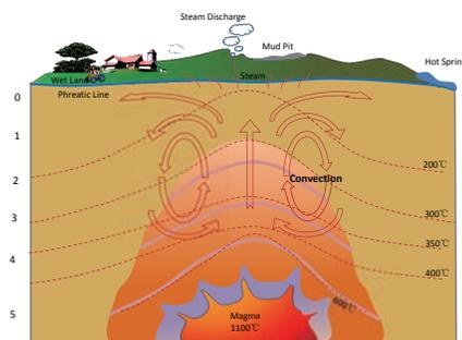
Schematic of an Ideal Geothermal System
