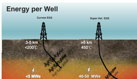
Different Power Generating Capacity of Different Enhanced Geothermal Systems (EGS)
